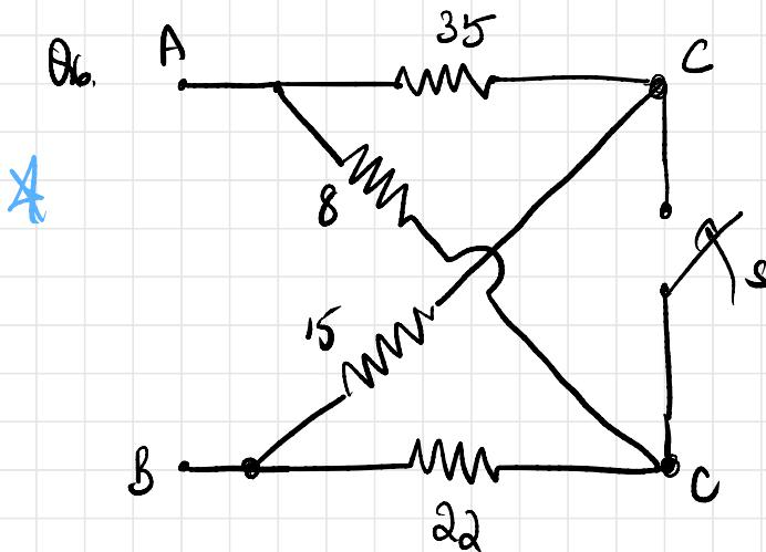
(i) For the circuit shown, find  $V_{AB}$  and voltage across  $R_2$  if switch S is open if V across is  $15 \Omega$  is  $45V$
