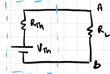
$V_{Th}$ : temporarily remove  $R_L$  and find open circuit voltage across load  $R_L$
